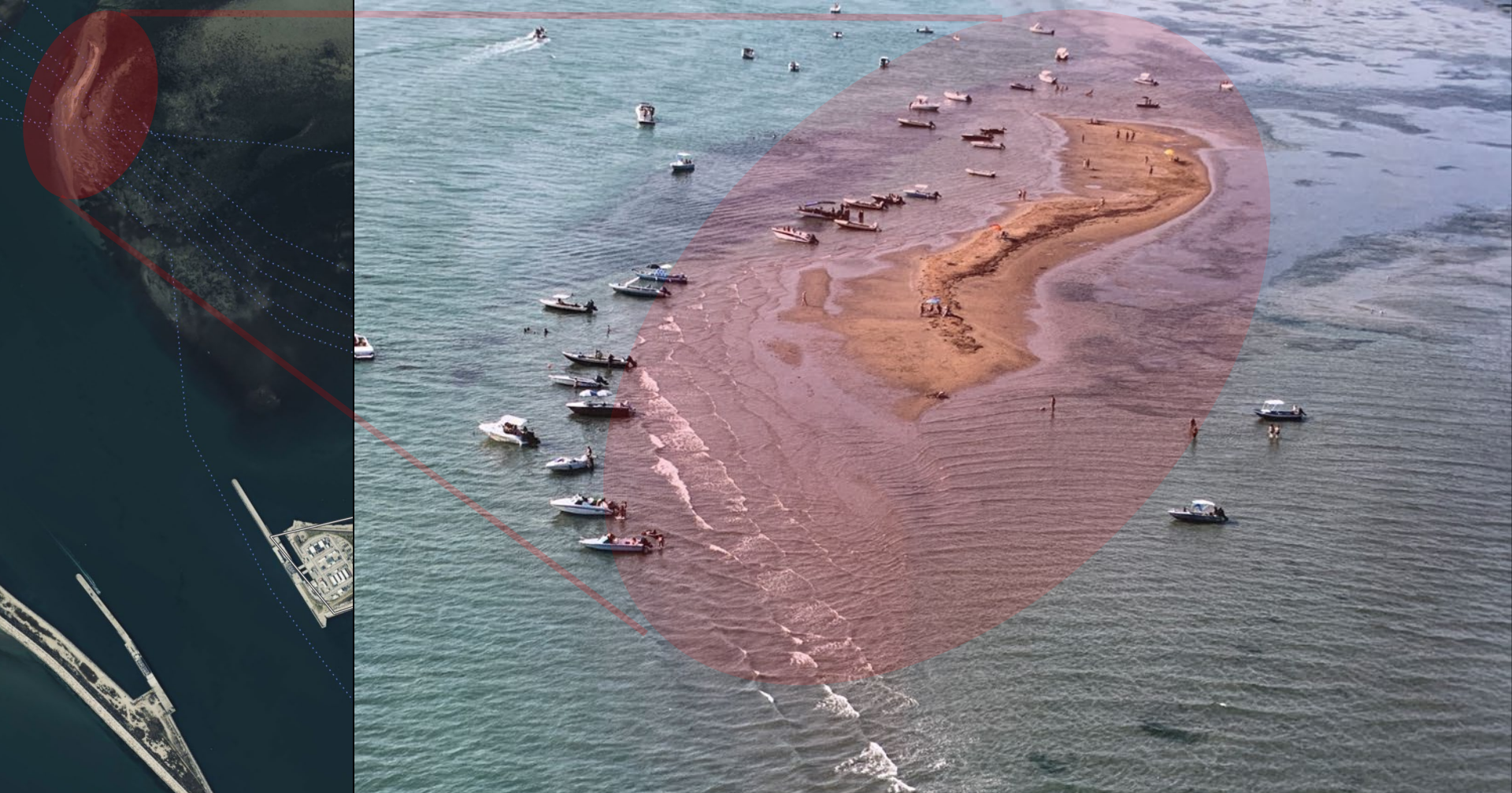
Unexpected new island induced by the Mose closures limiting winter shoal overtopping
