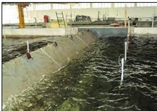
Foto 24 – Model of the bulkheads of Chioggia
