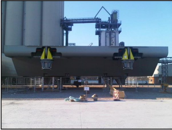
Foto 11 – Sluice gate with the two male hinge elements.
